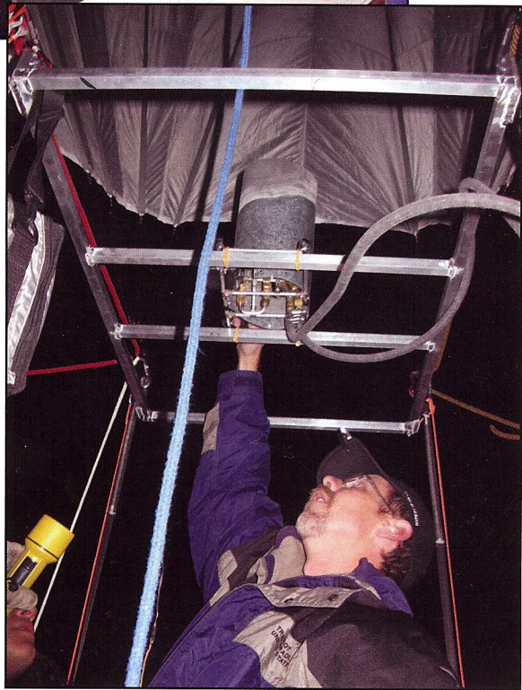
Checking the weather and lift calculations prior to launch, then a final pre-flight check of the burner.
